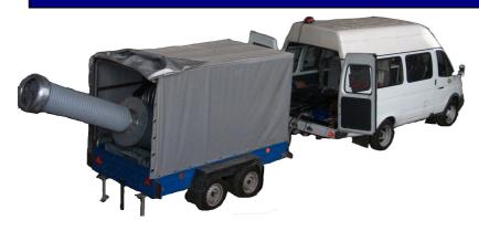
Gas-filled mobile test installation UVPG-250 is designed for tests of electrical equipment insulation with power frequency voltage of up to 250 kV inclusive. Owing to a low level of self- partial discharges (PD) it can be used for testing insulation with PD measurement at voltage of up to 200 kV inclusive.
